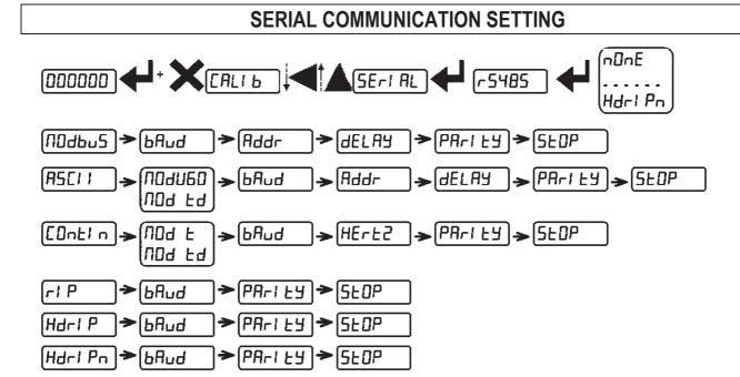
According to the chosen protocol only the necessary settings will be displayed in sequence (see diagram here above).
