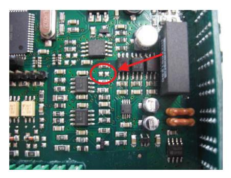
close the jumper shorting the pads with a drop of tin.
